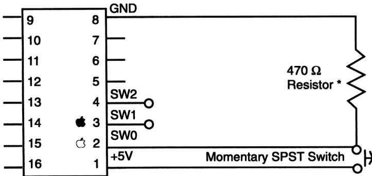
Apple IIe, IIc, and IIGS — External D-type miniature connector on the back of the computer, labelled with a small paddle icon.
